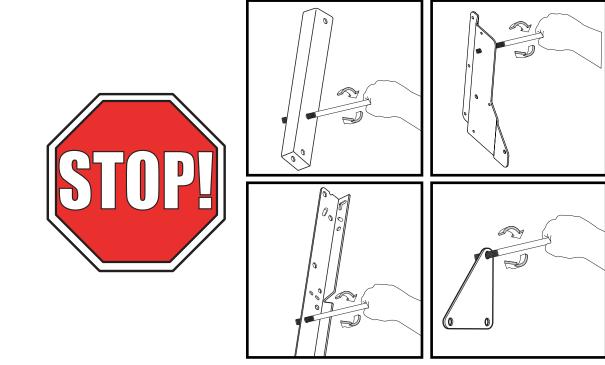
To ensure optimal playability of backboard system, a close tolerance fit between the elevator components and hardware is required. Test-fit large bolts into large holes of elevator tubes, backboard brackets, and triangle plates. Carefully rock them in a circular motion to ream out any excess paint from holes if necessary. Not all parts shown are included with every system.
